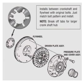
\*NOTES: The shim pictured "Full Sized" below can be used to make sure you select the correct shim. Just print these instructions and match hole pattern to flywheel. Be sure your printer is set to "No Size/Scale Change". You can check for correct scale by matching the ruler on the page.
