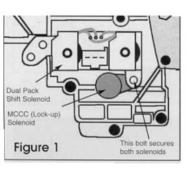
2. To Install: Insert the Dual Shift Solenoid into the valve body (Figure 1). Check the Resistance Test Locations (Figure 2). VPWR+ to SS1 resistance is 20 to 25 ohms. VPWR+ to SS@ reisistance is 20 to 25 ohms. Tighten the bolts to specification. Plug the OEM harness connector into the center of the new dual solenoid.
